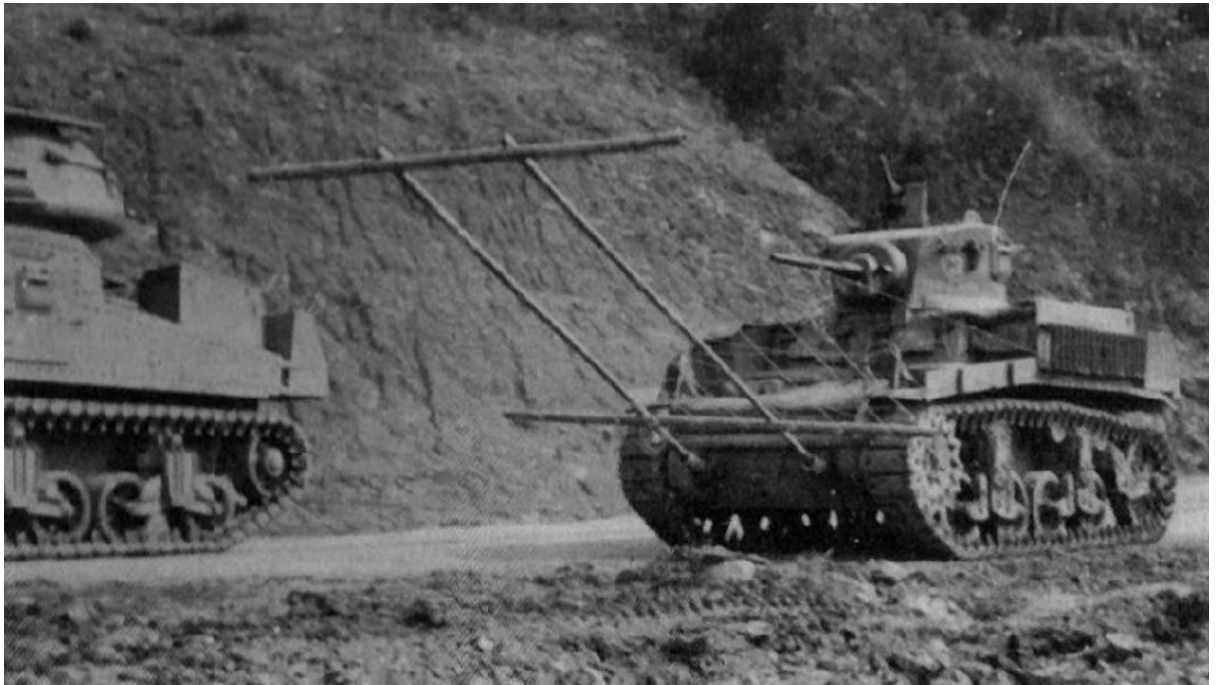
Above: On the left of this photo, taken at Kohima, is a Grant Mk I (note the turret shape) of 149th RAC. This regiment's RHQ, 'A' Sqn and 'B' Sqn were equipped with Grant, while 'C' Sqn was in the Arakan, equipped with Sherman Mk V. The Stuart is an attached 'minesweeper' tank belonging to 45th Cavalry (see XXXIII Corps below).
